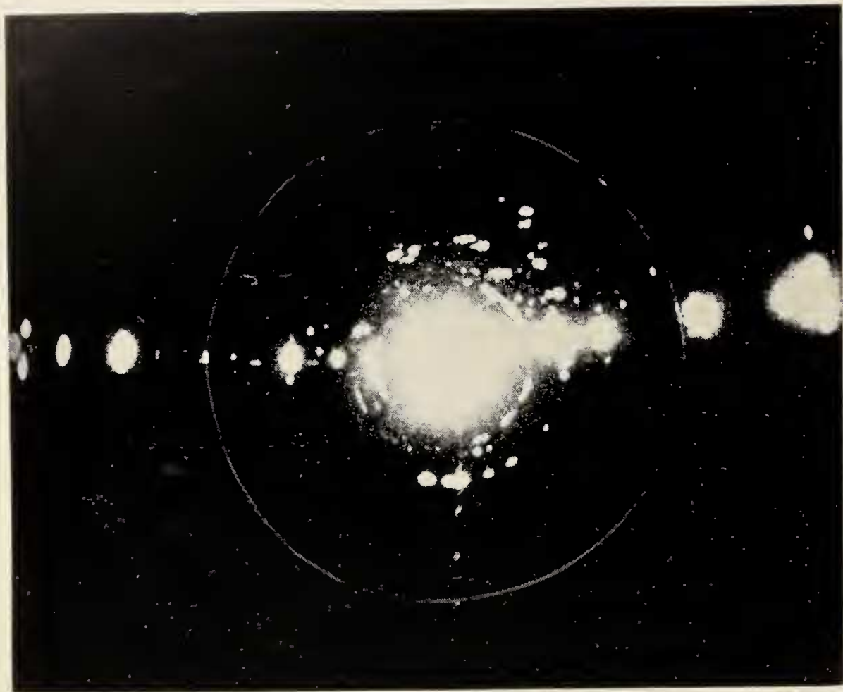
FIG. 3. Enlargement of a one-minute exposure of a 16-mm-radar-film frame showing presentation on radar indicator (scope) with antenna on 90^\circ (vertical) scan. Circle indicates two nautical miles from radar antenna. Large white marks to left and right of center are ground targets showing actual horizon. White spots above horizon are passerine birds. White spots below horizon are ground targets from spurious radar beams deflected from roof of radar building.
